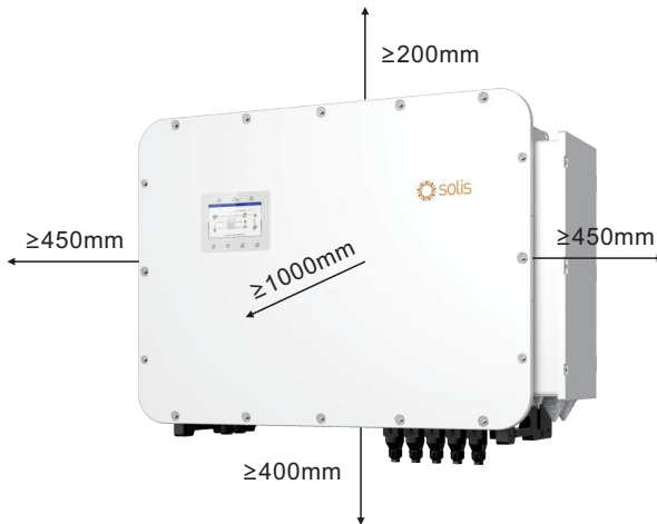
Figure 3.5 Inverter Mounting Clearances
