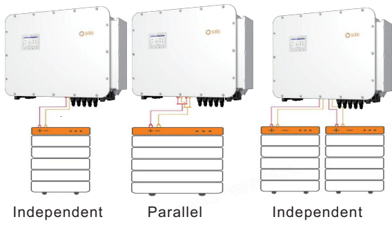
Figure 3. 20 Battery connection types
